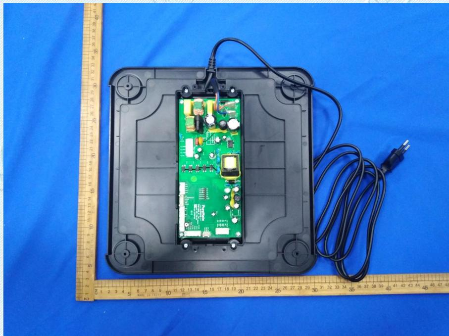
Photo 8- Internal view of PCB box
